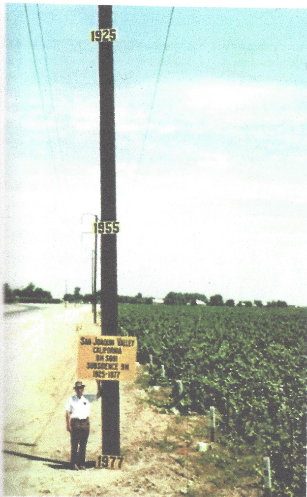
Figure 13-15 This pole shows subsidence from overpumping of an aquifer for irrigation in California's San Joaquin Central Valley between 1925 and 1977. In 1925, this area's land surface was near the top of the pole. Since 1977, this problem has gotten worse.
